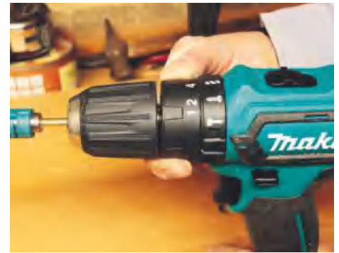
Dual collars on the drill make it simple to swap between drilling and torque driving
